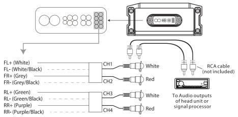
NOTE: In this connection, the AUTO POWER ON switch is in the OFF position.
